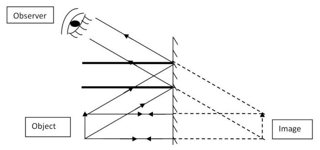
Figure 3. Ray diagram for image formation of an extended object
