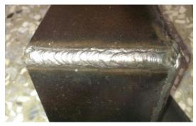
Figure 19. Welded Polish and Grinding
